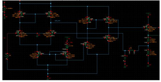
The region analysis shows the size settings of the NMOS and PMOS are appropriate, because the transistors are working at saturation region. The open loop gain reach to 35 dB, as shown below:
