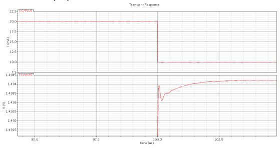
The plot shows that it takes time for the LDO to response to a load current step. The current initially comes for capacitor, hence the output drops. Once the LDO current equals the load current the output voltage stops decreasing. The LDO current then charges the capacitance. This overshoot happens because the compensation design.
