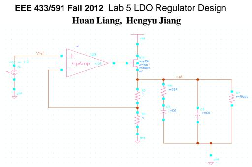
The LDO Poles and Zeros are the function of output capacitor ( $C_0$ ), the equivalent series resistance (ESR) of the output capacitor, and the bypass capacitor ( $C_b$ ). To decrease the voltage variation resulting from the load transient, a big value of output capacitor and the low ESR of the capacitor are selected as following table:
