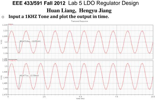
The output follows the input current with no phase change. The amplitudes of input and output are almost at the same values, which proves the feedback loop effectively regulate the output voltage.
