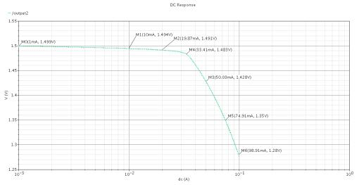
From the V<sub>out</sub> vs I<sub>load</sub>, the % change in Vout from **1mA to 33mA** is (1.483-1.499)/1.499 =**1%**. However, once the current goes above 33mA, it drops dramatically, (1.28-1.499)/1.499=**14.6%**
